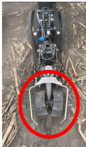
Figure 1. Dual dribble tubes on planter
