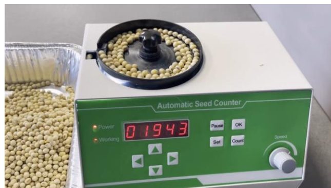
Figure 2. Soybean Seed Counter
