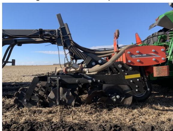
Figure 3. KUHN Krause strip-till unit
