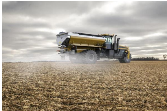
Figure 2. Strip-Till Banded Fertilizer with Montag cart
