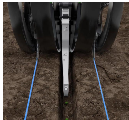
Figure 2. At-Plant Conceal Dual Band Nitrogen
