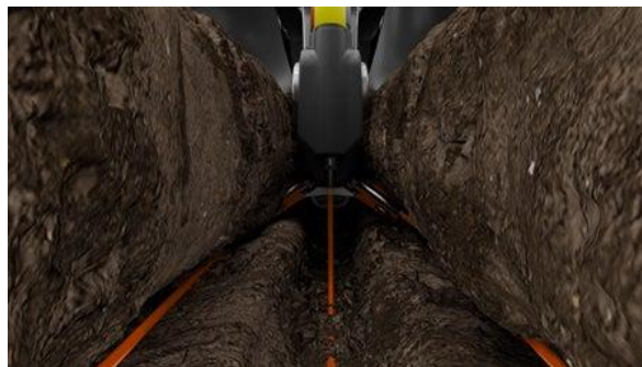
Figure 2: FurrowJet® Dual-Band Wings Fracturing Side-Walls
