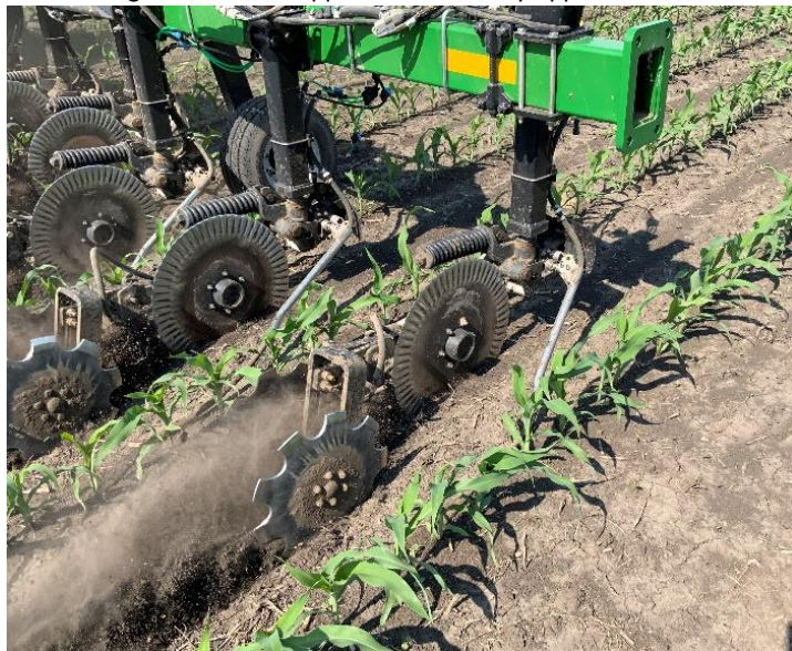
Figure 5. Surface Applied Dual Delivery Application
