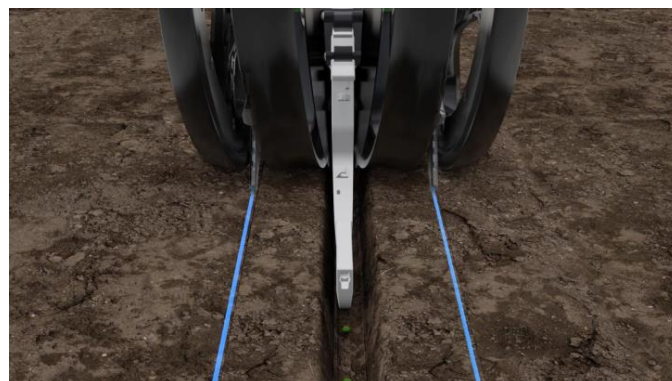
Figure 2. Conceal® Dual Placement 3" from Seed Trench
