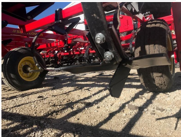
Figure 3. Finish™ Line Sweeps on 9" Spacing
