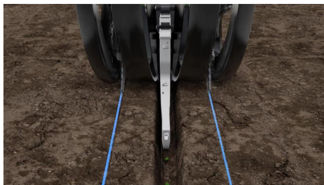
Figure 7. Conceal® Dual Placement 3" from Seed Trench
