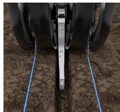
Figure 1. Conceal® Single or Dual Placement 3" from Seed Trench, 1.5" in Depth
