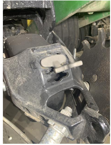
Figure 4. Reveal™ Depth Adjustment in Notch 1
