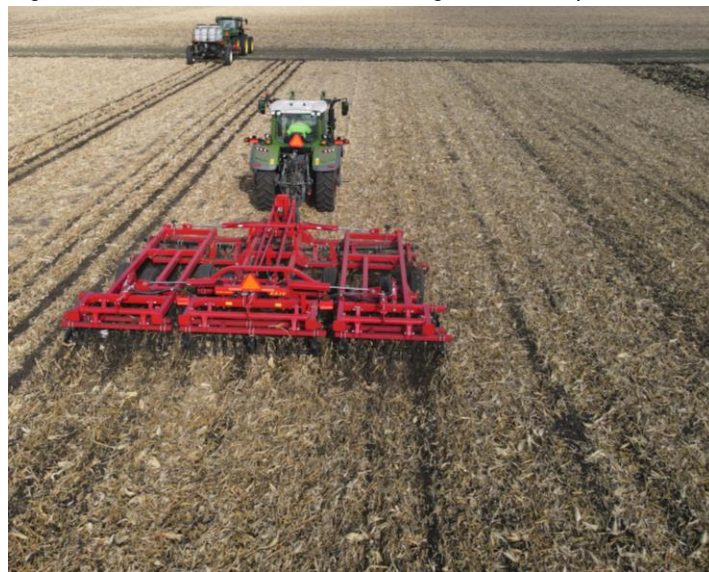
Figure 1. Sunflower® 6833 Vertical Tillage Before Strip-Till
