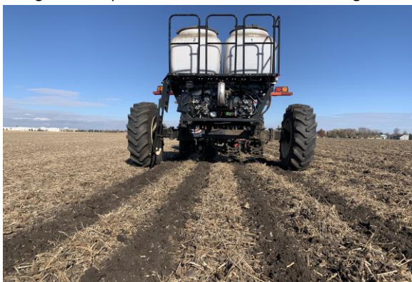
Figure 3. KUHN Krause strip-till unit
