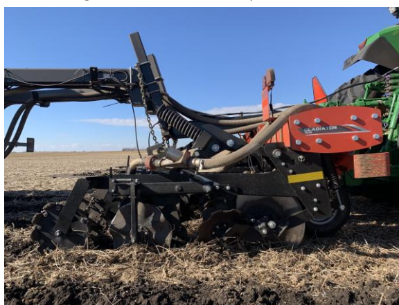
Figure 3. KUHN Krause strip-till unit
