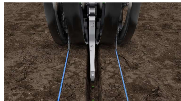
Figure 3. Conceal Dual Placement 3" from Seed Trench
