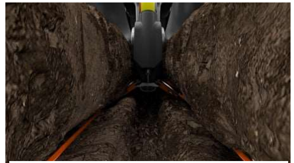
Figure 2. FurrowJet® In-Furrow Planter Attachment
