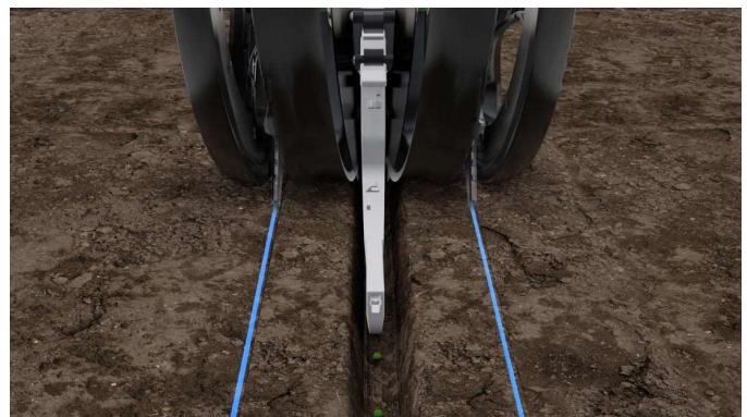
Figure 2. Conceal Dual Placement 3" from Seed Trench
