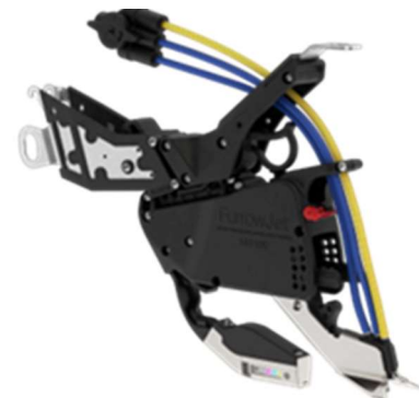
Figure 5. Conceal Dual Placement 3" from Seed Trench
