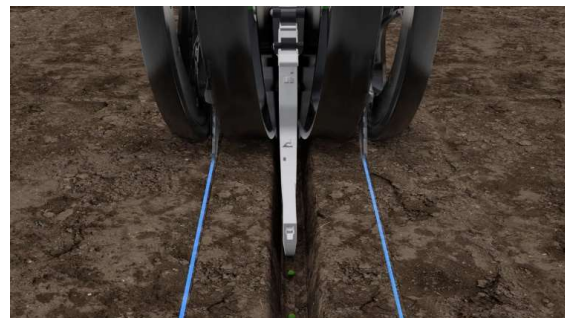
Figure 5. Conceal Dual Placement 3" from Seed Trench
