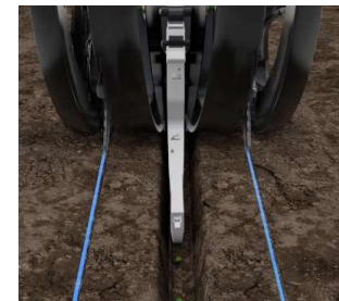
Figure 2. Conceal Dual Placement 3” from Seed Furrow, 1.5” in Depth
