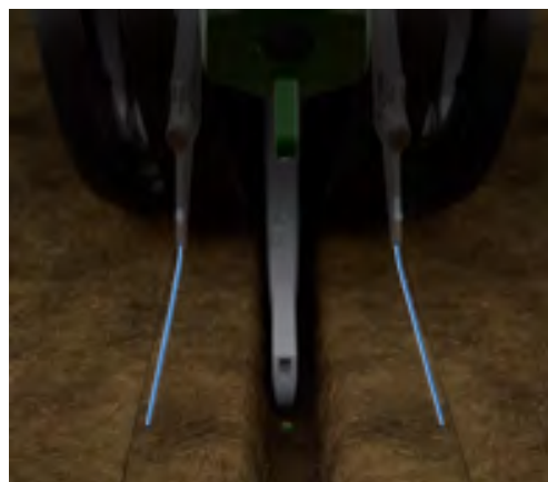
Figure 1. Conceal Single or Dual Placement 3" from Seed Trench, 1.5" in Depth
