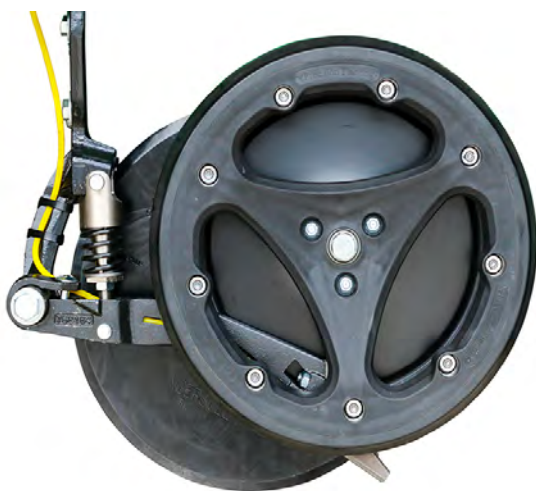
Figure 1. Conceal Knife Design within Gauge Wheel
