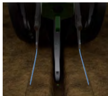
Figure 2. Conceal Dual Placement 3" from Seed Trench, 1.5" in Depth
